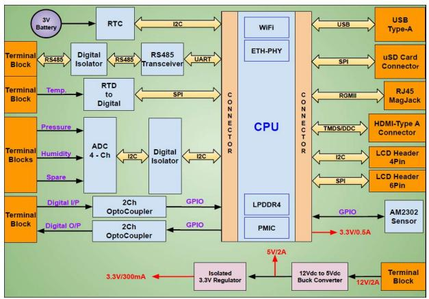
In our design system consists of a CM4 CPU running at 2.6Ghz, with 4GB LPDDR4 RAM, 32GB eMMC, 32GB SD card with built-in Gigabit ethernet, WiFi, RTC and digital/analog IO ports (4/8). The System is running on the latest version of Linux OS.
